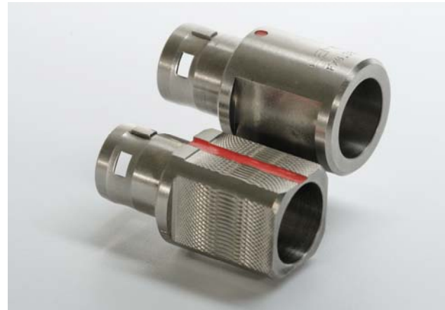
FIG Straight plug for remote handling, key (G) or keys (A...L and R), special alignment mark, knurled handling surface, cable collet
